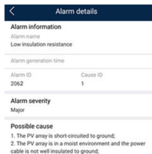
Figure D-1 Alarm details
